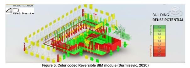
Figure 5 illustrates the results of Reversibility Assessment and Reuse Potential of building elements indicating material streams and reuse options through colour coding. A colour scale from red to green enables to respectively visualise the components with a poor or high reuse potential.
