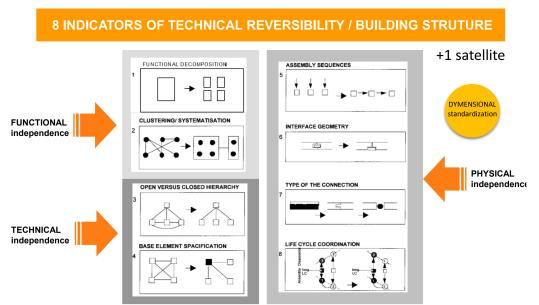
Figure 3. Indicators of technical reversibility of building being a part of Reuse Potential and transformation capacity calculation (Durmisevic, 2006)
